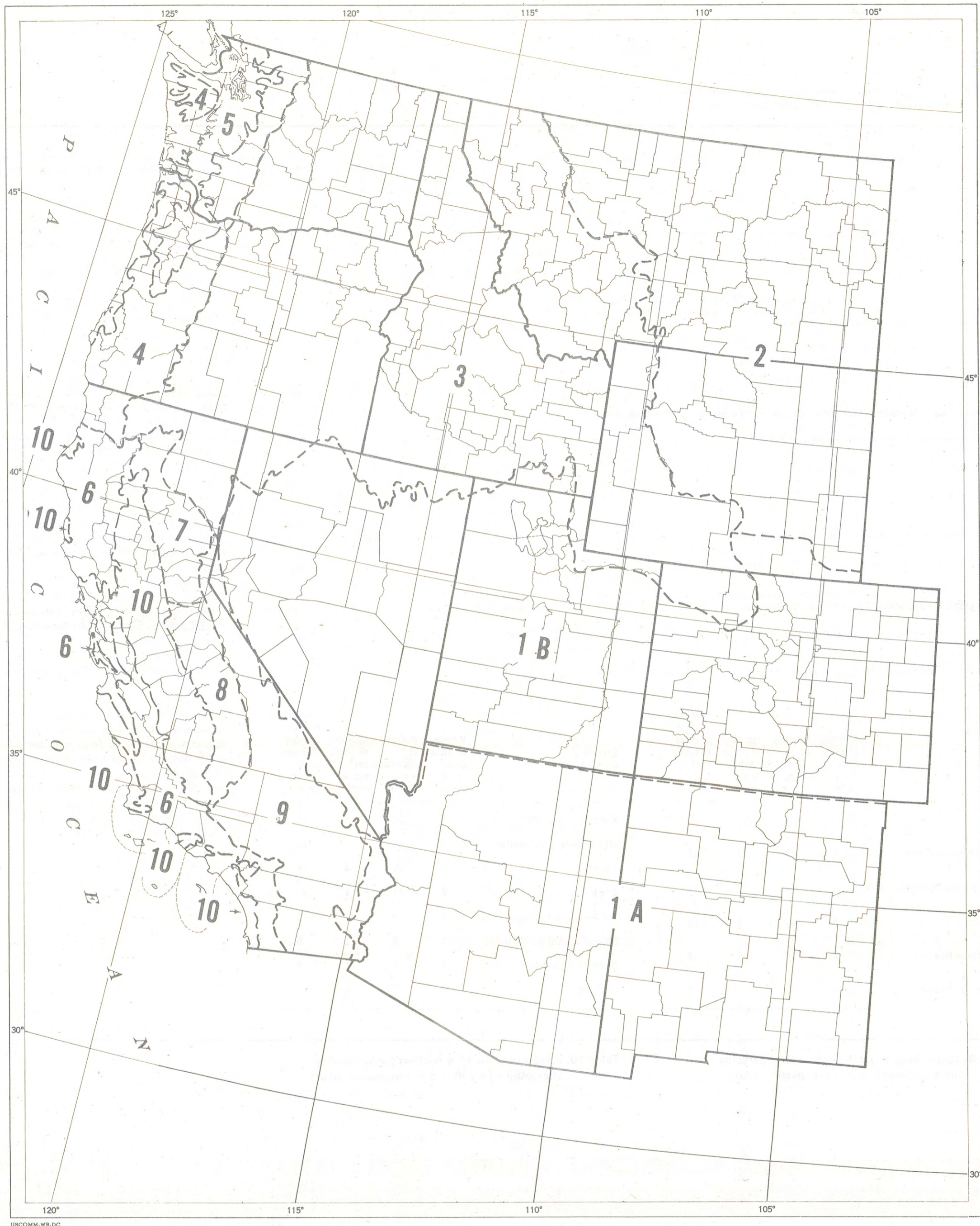
Figure 10. Regions used to develop statistical parameters for interstation interpolation of 2-yr and 100-yr 6-hr precipitation values.
